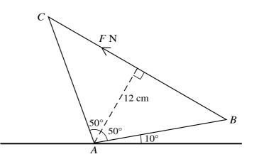
A uniform lamina *ABC* in the shape of an isosceles triangle has weight 24 N. The perpendicular distance from *A* to *BC* is 12 cm. The lamina rests in a vertical plane in equilibrium, with the vertex *A* in contact with a horizontal surface. Angle  $BAC = 100^{\circ}$  and *AB* makes an angle of  $10^{\circ}$  with the horizontal. Equilibrium is maintained by a force of magnitude *F* N acting along *BC* (see diagram). Show that F = 8. [3]
